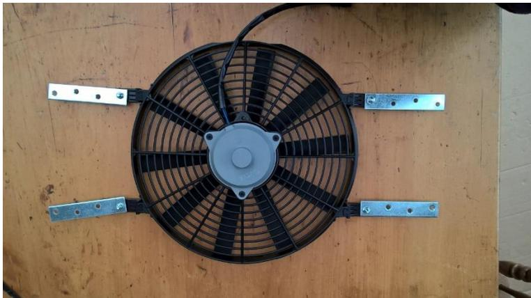
Next, by placing this assembly over my template (on the cardboard as shown previously) I was able to tighten the nylocs so that the mending plates were correctly oriented over the mounting points.
