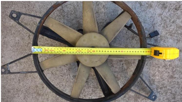
Shroud measured just under 400mm which meant that a 16 inch replacement was too big so purchased a 14 inch Calibre thermo fan.
