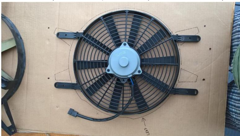
So, the next step is to make brackets that will extend to fit the 90. First, though, I test fitted the Calibre behind the radiator to check the space and found that the lugs on the Calibre brackets were fouling the radiator edges which meant they need to be shortened. This was done by removing the
