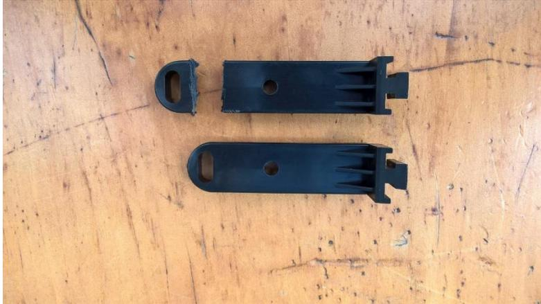
In order to get my brackets fastened to the Calibre mounts as securely as possible, I drilled a 6mm hole in each plastic mount between the 2 extended lugs on the other side of the plastic mount as in next picture:
