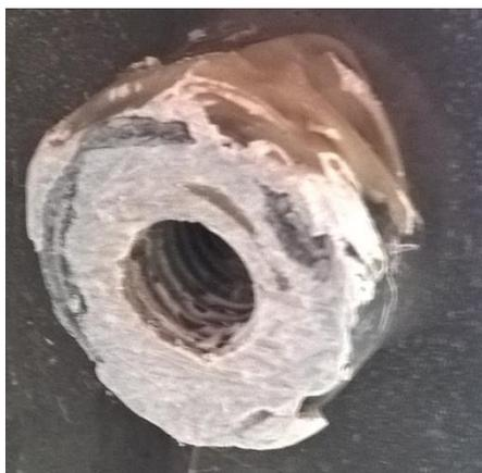
Finally, you can clean up the remaining excess plastibond around the outside of the boss if you want a really neat finish. I just rasped back to the boss face and left the rest (once the spoiler is refitted it can't be seen).
