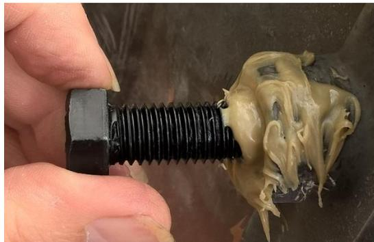
This looks messy but don't worry, you can clean up excess later. The main thing now is to hold the bolt in place and as square as possible for about 4 minutes to allow the plastibond it's initial set. Viewing the bolt from the top down will help you set it square to the boss.
