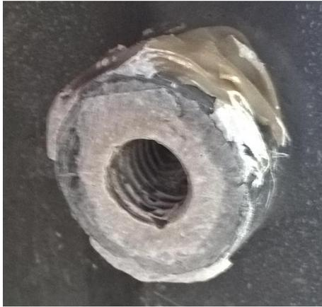
To clean up the thread before refitting, you can just screw in the 14mm bolt and then remove it.
