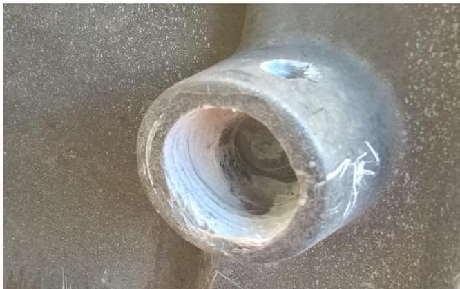
You will also note that the boss has 2 additional holes drilled through its sides almost opposite each other. These are to create a "key" in the 2 pack which will give it additional strength and lock it into the existing boss. A 5 or 6mm drill bit will give you a large enough hole without destroying the integral strength of the boss.
