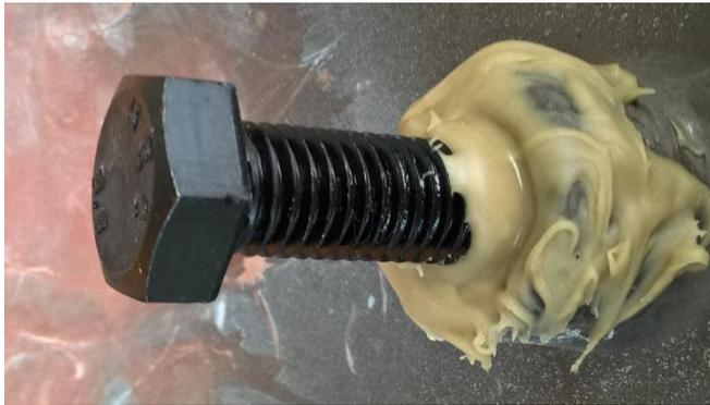
Leave it until the plastibond has completely cured and hardened.
