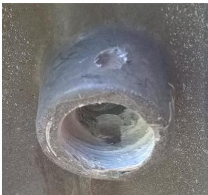
As the thread you want is 14mm (I measured the captive bolt that fastens into this thread) get a 14mm bolt around 50mm long and coat the lower half of the thread with Vaseline:
