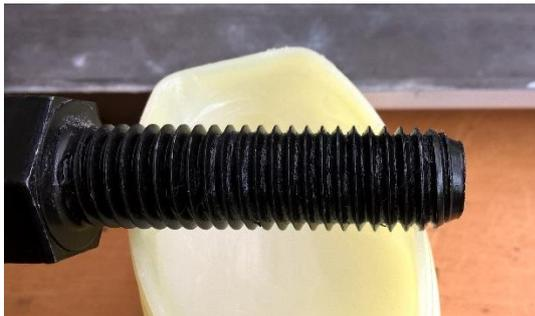
Next, mix enough of the Plastibond to fill the cavity you've created in the boss and quickly put a thick coat of the Plastibond on the end of the bolt and put the remainder of the bog the into the hole in the boss, making sure that it goes into the 6mm "key holes". Then insert the bolt into the hole in the boss:
