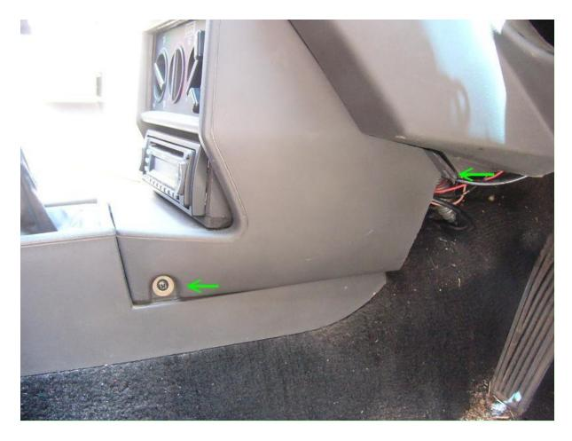
Step Slide the main console towards the rear as far as you can to disengage the hook under the heater console.
