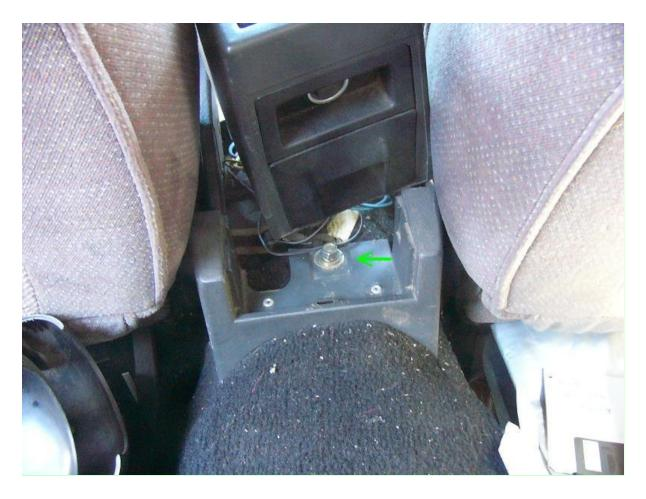
Step 4: Remove the four screws (two either side) holding the heater/radio console.
