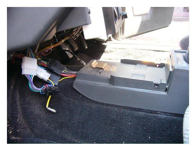
Step 6: Remove the heater/radio console, disconnecting the radio wiring as you go.
