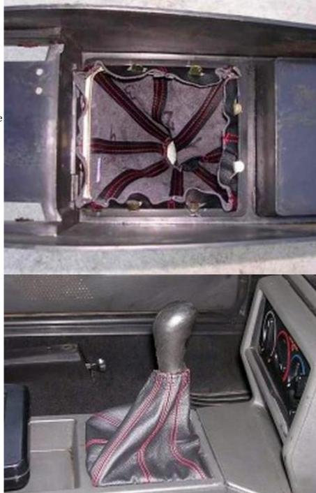
**13.** Place the new boot into the console from the top. Turn the console over and bend the tabs over to secure the boot to the console.
