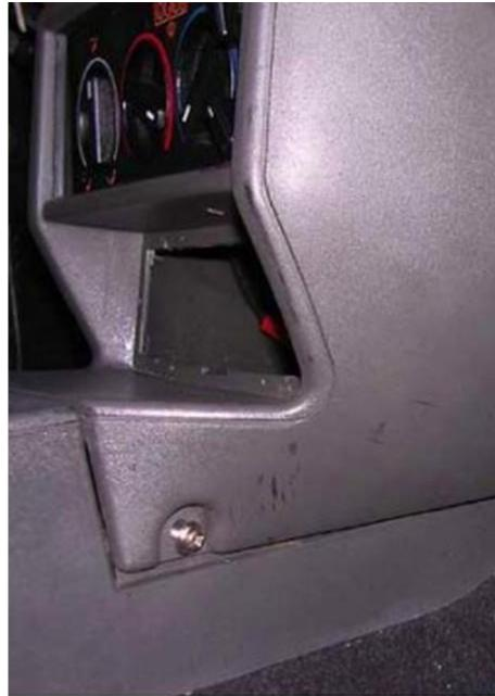
3. Remove the four trim screws holding the center stack in place. There are two attaching the center stack to the console and two attaching the center stack to the firewall.
