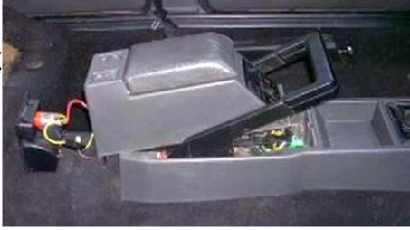
**5.** Remove the #12 bolt holding the console to the transmission tunnel.
