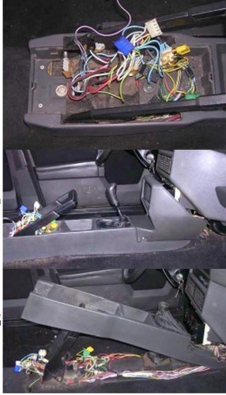
8. Here is a detail of the center stack and console after removal. You can clearly see the plastic tabs where the stack is screwed to the firewall and tabs that slide into instrument panel. Note the metal clip on the console and the wire rod on stack. Sliding the console to the rear releases the clip from the wire rod and allows the stack to be separated from the console.
