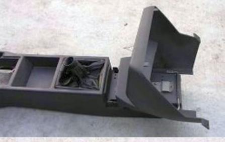
**9.** To remove the boot, turn the console upside down and bend the clips where they are wrapped around the plastic. The old boot will now be free to be removed from the top.
