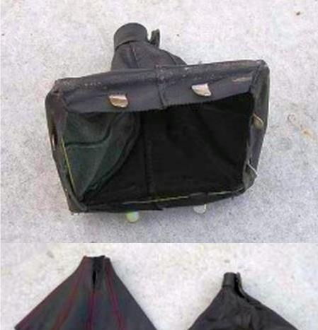
**10.** Here is the new boot compared to the old. Remove the metal retention ring from the old boot.
