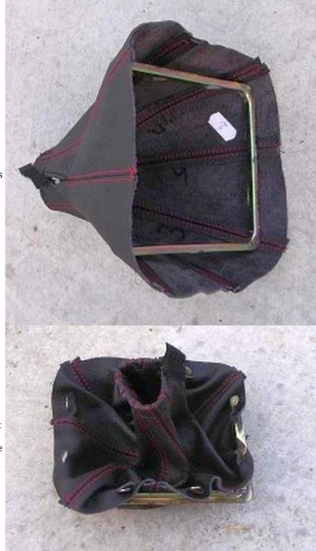
11. Install the retention ring into the new boot. Make sure to orient the ring the same way it was on the old boot.
